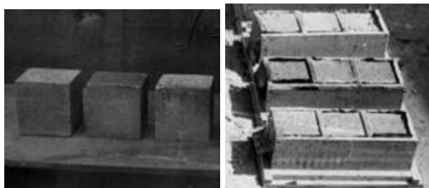
Figure 3. Concrete samples depending on the method of care; t = 43^{\circ}\text{C} , \alpha = 35\% , project brand of concrete-300.
