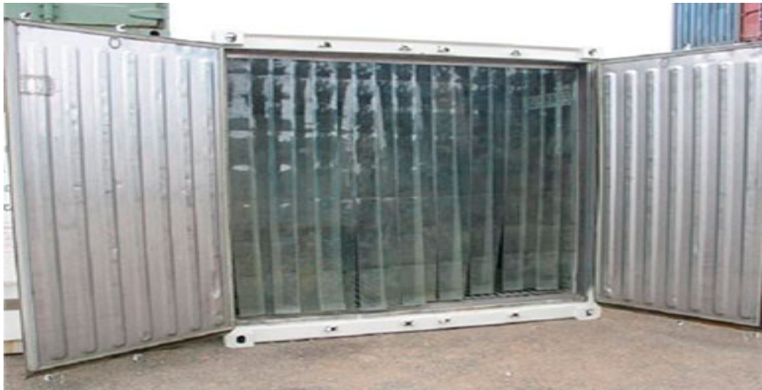
Figure 17. PVC curtains on the door.
