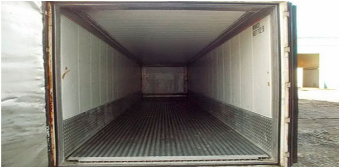
Figure 12. Wall structure of a 40-foot refrigerated container.
