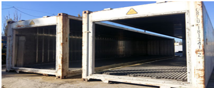
Figure 11. 40ft Refrigerated Container Frame Structure.
