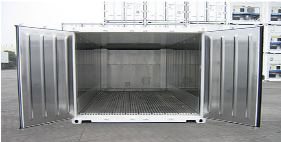
Figure 15. Door part structure of 40ft refrigerated container.
