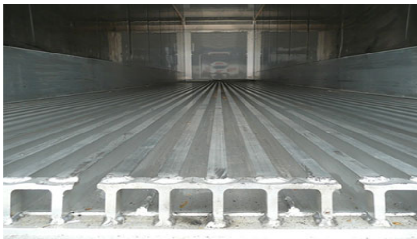
Figure 13. The floor structure of a 40-foot refrigerated container.
