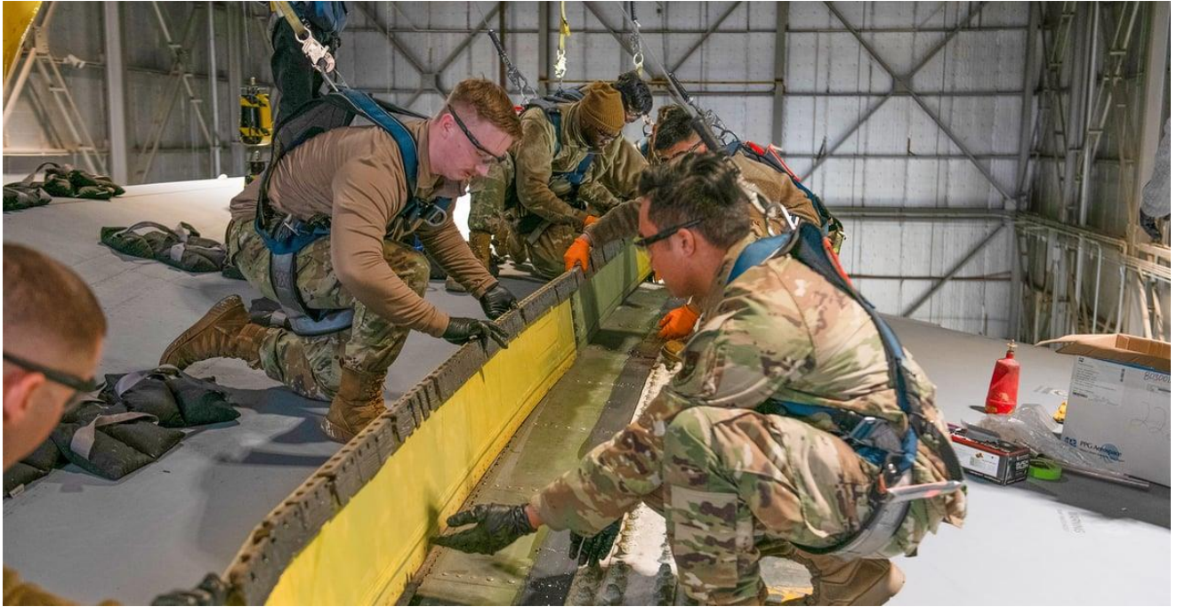
Figure 6 Solders making repair incorporating 3D-printer parts [12].
