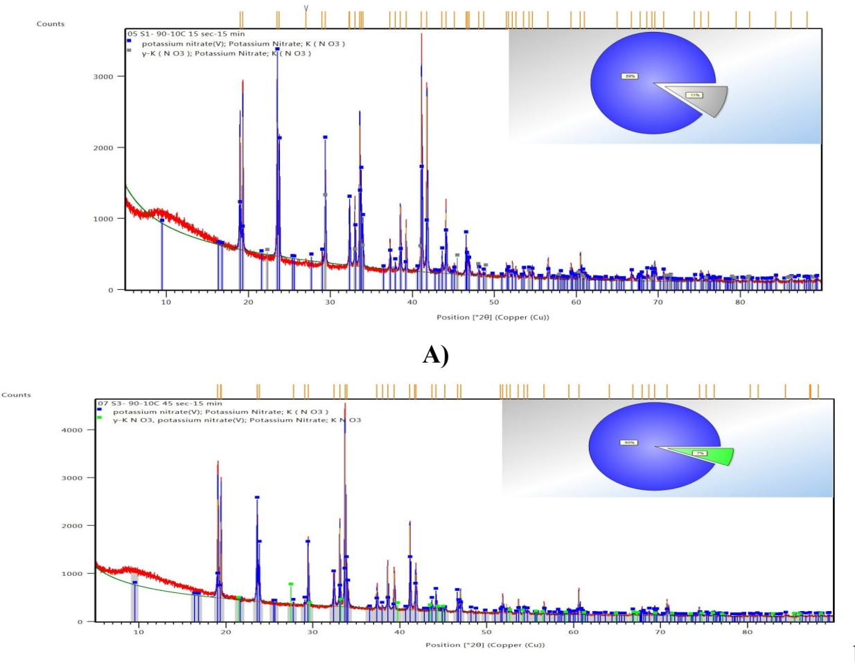
Drawing. X-ray patterns of potassium nitrate obtained at the time of exchange decomposition, (min): a-15; b-30.
