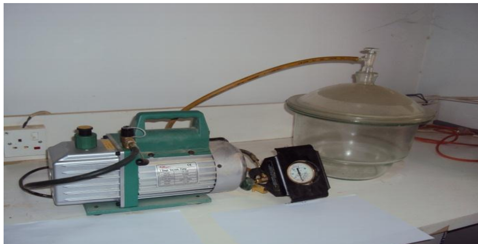
Figure (3-6) Vacuum pump and model container.
