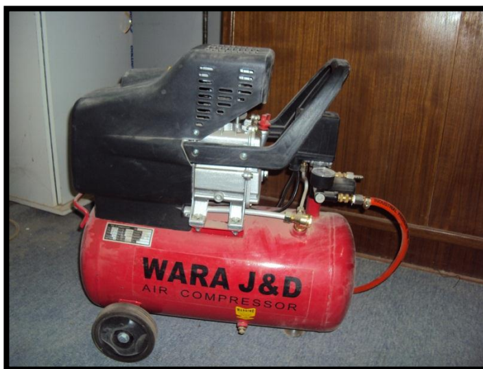
Figure (3-5) Compressed air pump.
