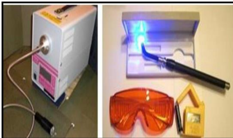
Fig 2.5: Left a UV (308 nm) light for the treatment of psoriasis; (Right) a pen-type blue laser (at 405 nm) for the treatment of acne.
