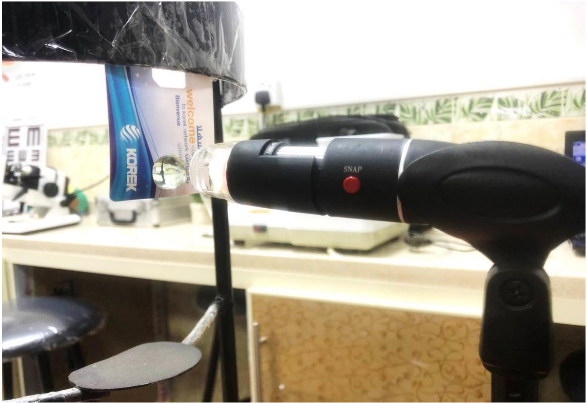
Figure 3.8: Image taken from a glass ball of known radius for normalization process
