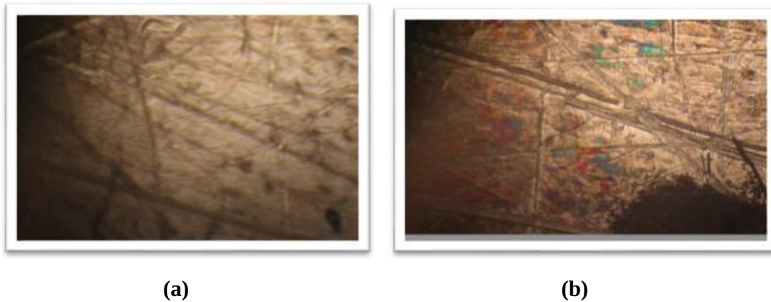
Figure (3.5): microscope image for silver (a)before laser (b) after laser effect
