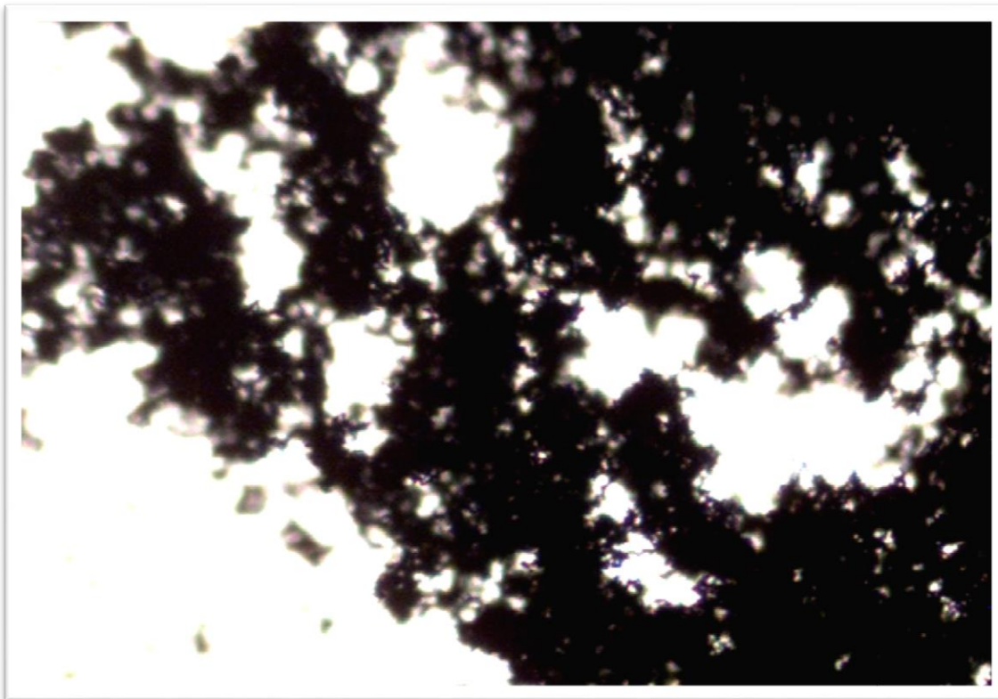
Figure (3.8): Microscope image for cobalt powder
