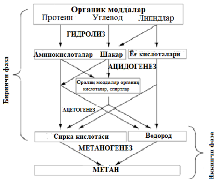
3 - Picture. Decomposition steps of an anaerobic converter
