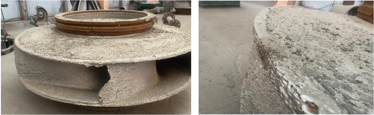
Fig. 3. Wear of the inlet parts of the blades
