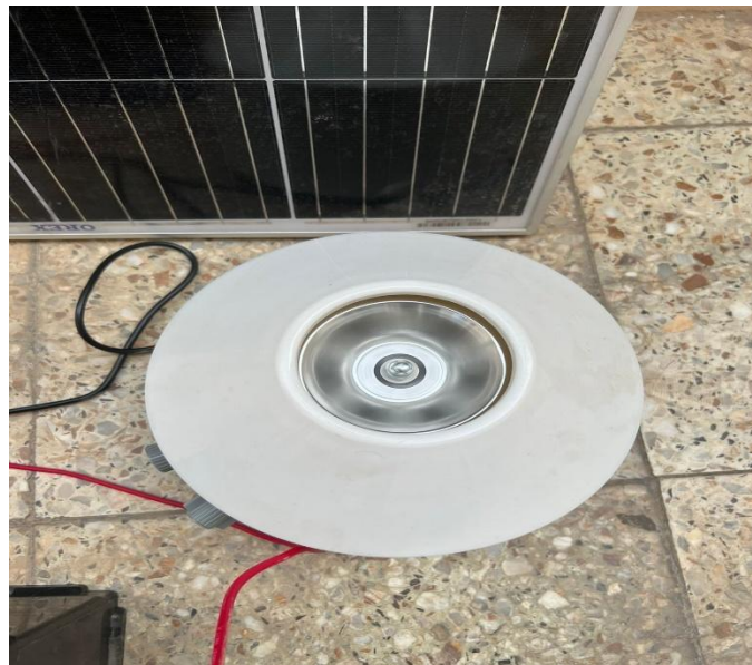
Fig:4-4 centrifuge working at 220 dc voltage
