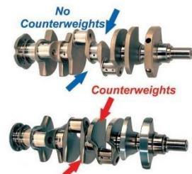
➤ **Periodic Forces:** The repetitive motion of engine components results in periodic forces that propagate through the engine structure. If not synchronized, these forces can resonate, leading to severe vibration and noise. Advanced balancing techniques aim to align these periodic forces to cancel each other out, reducing their overall impact on engine stability.
