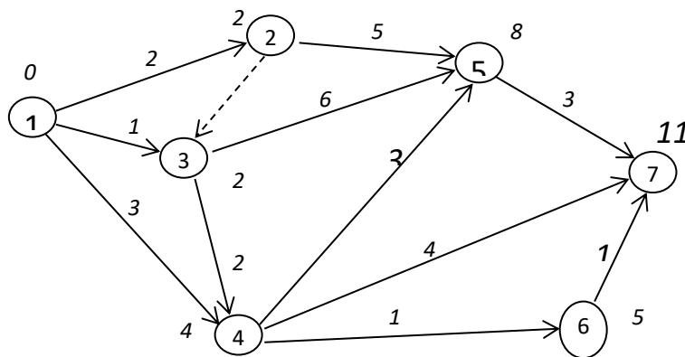
First we find the expected (early) time of occurrence of  $t_i$ ,  $i = \overline{1,7}$ , events. It will be as  $t_1 = 0$  agreed. Only operation  $R_{12}$  leads to event 2, and since the execution time of this operation is  $t_{12}=2$ , the early time of occurrence of event 2 is  $t_2=t_1+t_{12}=0+2=2$ .
