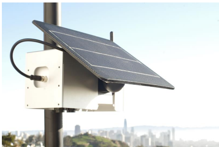
Figure 3: Low-cost, stationary sensors, such as the Clarity Node-S shown above, can be placed in a range of settings and provide high spatiotemporal data resolution local air quality data collection. [16]
