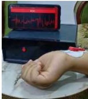
Figure 19. Patient Setup for ECG Signal Acquisition Using Electrodes The figure.
