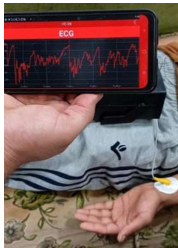
Figure 20. Real-Time ECG Visualization on Mobile Device via Bluetooth.
