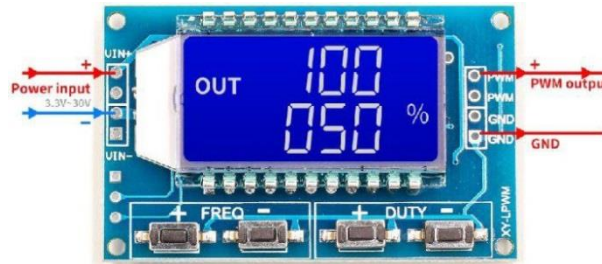
Figure 7. PWM frequency and duty cycle signal generator board with display
