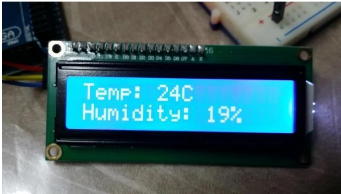
Figure 13. LCD Display Showing Temperature and Humidity
