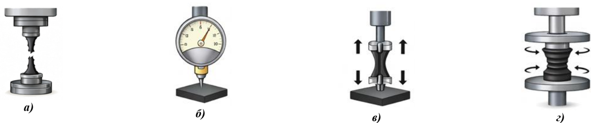
Fig. 3. Instruments for determining the technical indicators of filled vulcanizations: a) Rupture, device: IR-5 type rupture machine Standard: GOST 262-03 Measured characteristic: rupture resistance ( R_a ); b) Hardness (Shor-A) Device: Shor-A hardness tester Standard: GOST 263-03; c) Multiple stretching Device: IR-5080 type stretching machine Standard: GOST 270-95 Measured characteristics: conditional strength ( \sigma ), relative elongation ( \epsilon_{relative} ), residual elongation ( \epsilon_{rest} ); d) Fatigue compression. Device: Press with control load. Standard: SEV 121-78.
