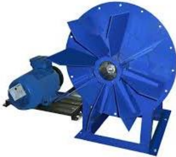
Figure 1.3. Straight blade centrifugal fan blade with disc
