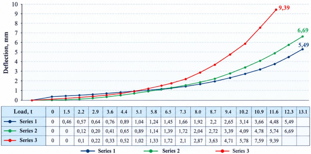
Figure 3. Comparison of vertical deflections measured by dial gauge D-5 (series 1 – M-1, series 2 – M-2, series 3 – M-3)
