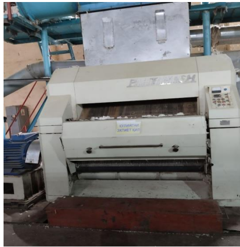
Figure 3. Production appearance of a 90-saw gin with an improved grate
