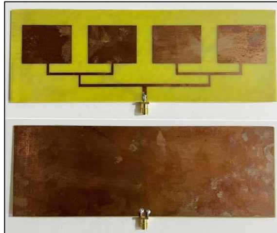
Figure 9. Front and rear view of the antenna array (4×1).
